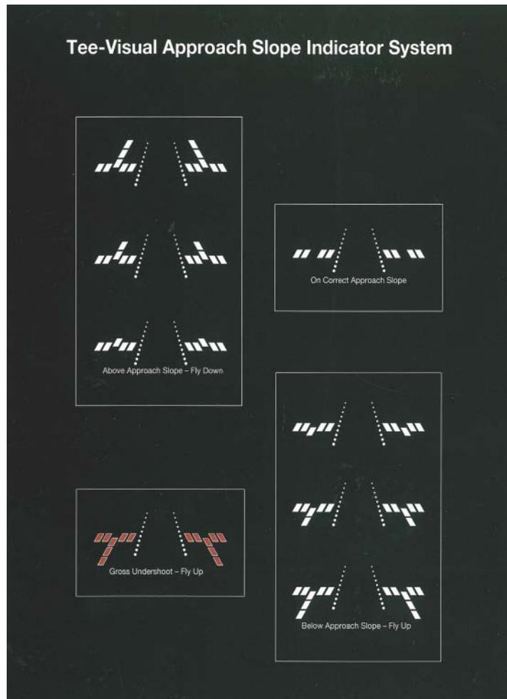
Figure 2: The Tee-Visual Approach Slope Indicator System runway light scheme
